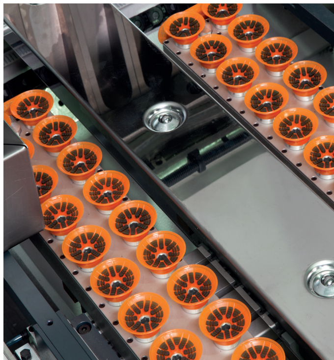
Suction plates in gauge table, controlled via POS 3000.
